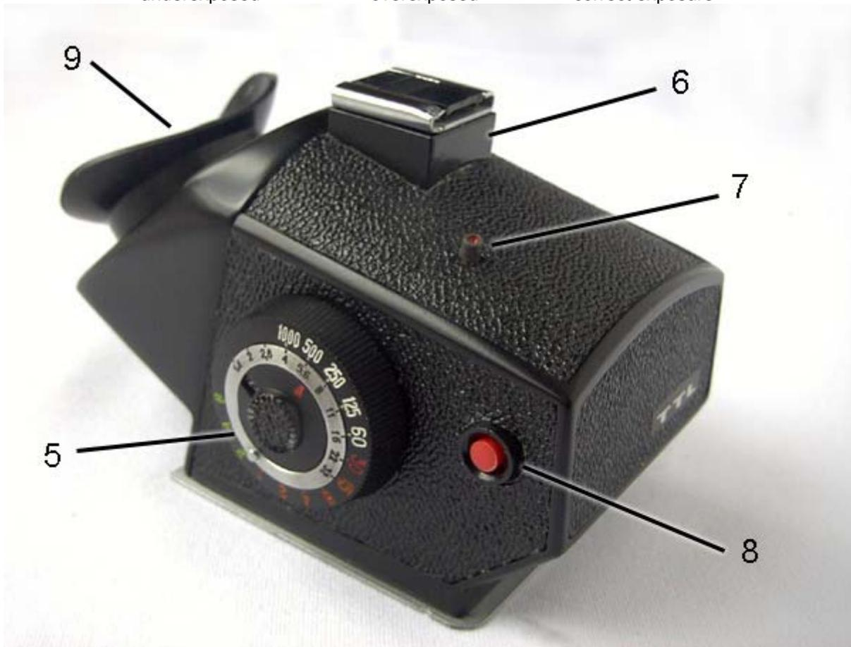
If you see the "underexposure" red LED, located on the left in the viewfinder field of view, slowly turn the exposure dial knob 1 counter-clockwise until the "correct exposure" green LED, located in the center, appears.
