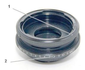
ARAX shift adapter allows you use any ARAX lenses on 35mm digital and classic camera including full-frame DSLR. It gives the 11 mm shifting possibility of lens and 360 degree rotation. The lens which you can use with this adapter should have KIEV-C (Pentacon Six) mount. It is a full range of lenses manufactured by ARSENAL factory (Kiev), Carl Zeiss Jena (Germany), other lenses with PENTACON-six mount. There are no problem with any lenses and infinity focus.
